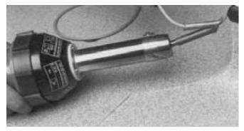
Groove the floor and bottom section. The top section of the mitre forms a natural 'Vee' and does not need grooving. Start welding the mitre from the top, with the weldrod feed above the nozzle. When welding the floor feed the weldrod below the nozzle.
